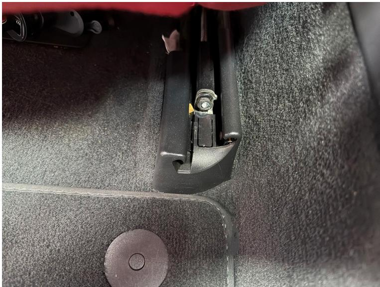
2. You will need an M10 triple square to loosen the seat bolts. Do NOT fully remove it. You only need enough space to splice the bracket under the factory bolt.
