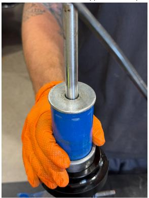
8. Install the top hat washer before reassembling the strut.
