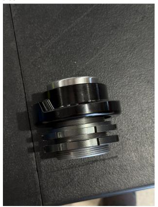
5. Lube the inner ring before installation.
