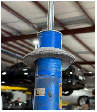
4. Assemble the TRP Coilover Sleeve Perch and verify that the rings are in the correct order.
