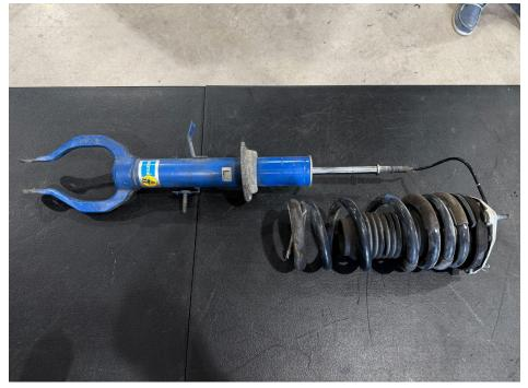
3. Press off the lower spring perch and remove it.
